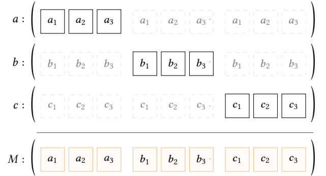
Figure 5: Visual representation of the WRAPUPREPEATED procedure; M is the resulting Row-major matrix
