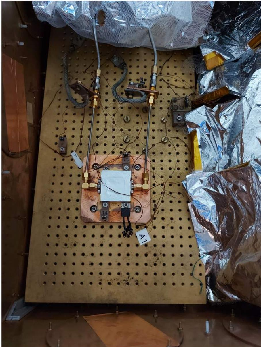
Figure 4.9: Inside of the cryostat, with all the cold component of the set-up.
