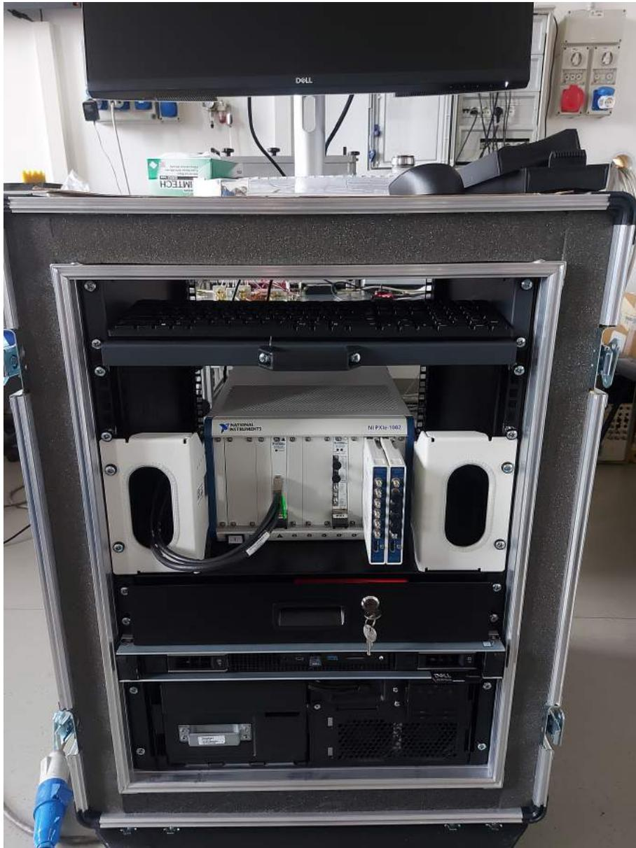
Figure 4.8: The insulated rack with all the warm electronic components.
