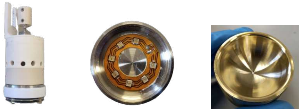
Figure 3. (Left): picture of the e-gun. (Center): anode with 7 LEDs used to illuminate the cathode and the aluminum cylinder with UV light. (Right): gold-coated cathode used to collimate the electron beam. The aluminum cylinder, where electrons are produced, is visible in its center.
