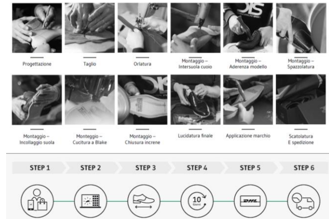
Fig. 4. Process of handcrafted men's shoe production and steps of mass customization strategy supported by FF MTO
