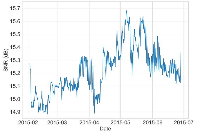
Fig. 1. SNR values over time of a single illustrative lightpath from the publicly-available Microsoft WDM optical backbone dataset. SNR values are averaged over windows of six hours.
