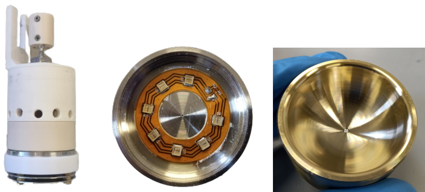
Figure 3. Left: picture of the e-gun. Center: anode with 7 LEDs used to illuminate the cathode and the aluminum cylinder with UV light. Right: gold-coated cathode used to collimate the electron beam. The aluminum cylinder, where electrons are produced, is visible in its center.
