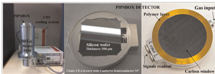
Fig. 2.4: a, Schematic of four major steps for production and analysis of atmospheric xenon sample by SPALAX-NG station (reproduced from Topin, S. et al. 10 ). b, Left, germanium/silicon (PIPSBOX™) radioxenon detection setup devoted to the SPALAX™NG (without the shielding); middle/right: gas cell of 11.7 cm 3 active volume equipped with two silicon detectors for electron detection and protected by a 600 \mu\text{m} carbon epoxy window entrance.
