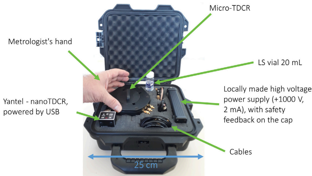
Fig. 2.7: The whole set of components, including locally-made high voltage supply, can be easily handled and connected to a portable computer. Reproduced from Sabot, B. et al 17 .
