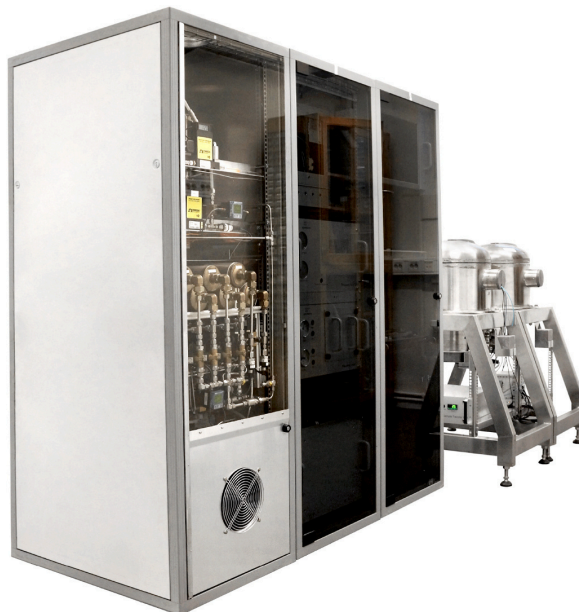
Fig. 2.3: A picture of the first SAUNA III system, with the two detector lead-shields in the back.
